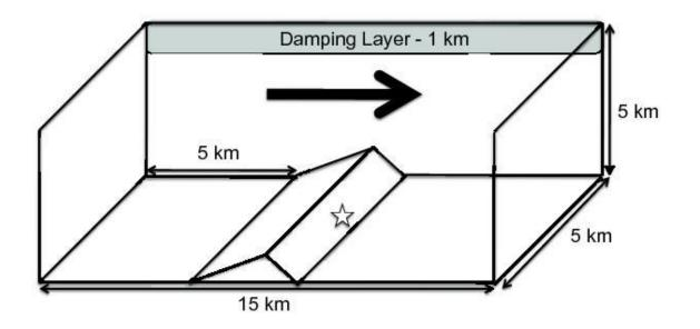
Figure 1. Model domain showing the triangular mountain with its ridge line oriented perpendicular to the input wind field. The windward slope is inclined at 20° and the leeward slope is inclined at an angle of  $\alpha^{\circ}$  ( $\alpha = 35^{\circ}$  in the first set of simulations and is variable in the second set of simulations). The star on the leeward slope indicates the approximate location of the ignition used in the simulations.
