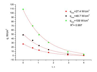
Figure 4. Heat flux versus time when the sample is moved from the focal plane
