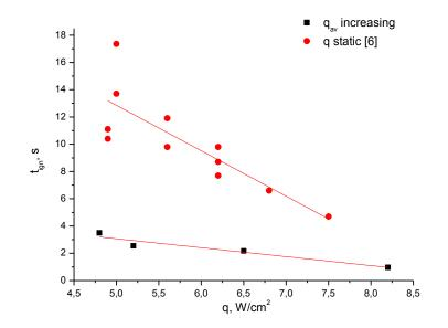
Figure 6. Ignition delay times of the pine samples versus heat flux for dynamic (increasing heat flux) and static conditions
