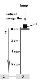
Figure 2. Installation for the movement of the sample: 1 is the sample, 2 is the remote control of motion platform with a sample; 3 is the mechanism that move the sample, y = 0 cm is the focal plane; 3, 5, 8 cm are the distances from the focal plane
