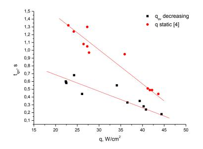
Figure 5. Ignition delay times of the pine samples versus heat flux for dynamic (decreasing heat flux) and static conditions
