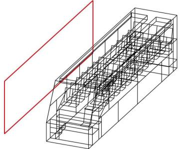
Figure 1. Scheme of a bus with 6 spaces, 99 main bodies, 105 interior bodies, 18 windows and 1 fire front.
