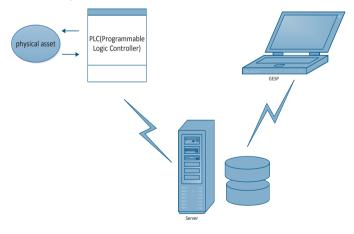
Fig. 3. Communication of the physical asset with the GESP application
