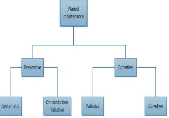
Fig. 4. Classification of planned maintenance in GESP application
