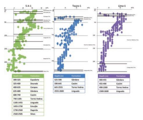
Fig. 4 – Porosities from wells 5A-1, Touro-1 and Lima-1 of Porto Basin. The values represented were obtained by reading a spacing of 5m.
