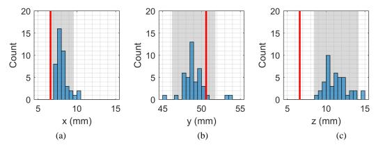
Figure 12 - Histograms of the measured dimensions of the 43 airborne sticks. Red lines: true stick dimensions; greyed areas: expanded uncertainties  $(\pm 1.5, \pm 2.8 \text{ and } \pm 2.9 \text{ mm for a, b and c, respectively})$
