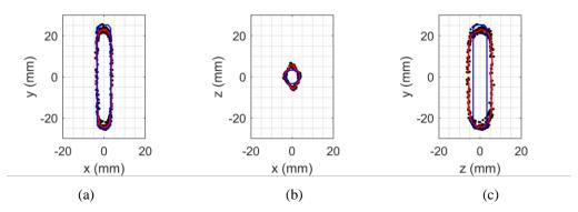
Figure 11 Orthogonal views of a reconstructed particle show good agreement, particularly in the x- and y-directions. Added length is observed in the z-direction due to lack of visibility of the back of particles, increasing the size of the visual hull.
