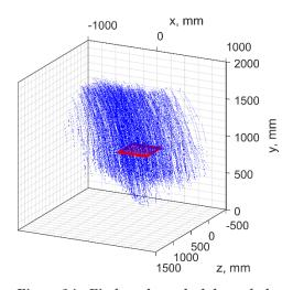
Figure 14 - Firebrands tracked through the control volume (N = 1032).
