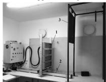
Figure 1 - Radiative Heat Flux Apparatus
