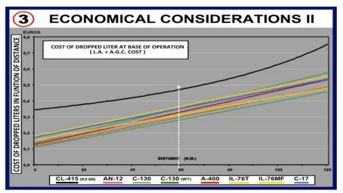
Figure 9: Cost of dropped water as a function of distance
