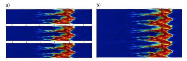
Figure 1. Top down view of 6 m s-1 wind 40 m wide fire simulation a) (in red dotted box) and the use of periodic boundary conditions to conceptually approximate an infinite-length fireline a) and b). In these images the colors indicate gas temperatures (Dark Blue is 300 K and red is greater than 1100K.) These images show the fingering behind the fireline and lobes in front of the fireline. This structure was ftypical for the infinite fireline simulations with 6 m s-1 and stronger winds.
