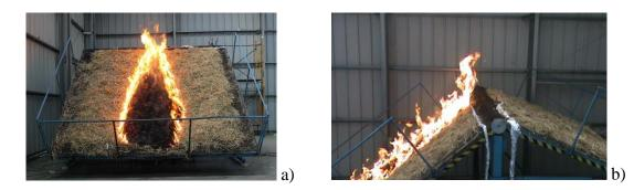
Figure 2. Picture of the test SE11 with parameters:  $\alpha_A = 40^\circ$ ,  $\alpha_B = -20^\circ$ , c = 0.30m. a) Front view, b) Side view with detail of the ridge and fuel break.
