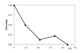
Figure 4. Average probability of fire crossing as a function of  $c/L_1$  for classes with a step of 0.13 between them.
