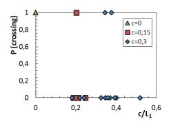
Figure 3. Probability of fire crossing as a function of  $c/L_1$  for all tests.
