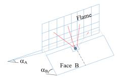
Figure 5. Skecth of the radiation flux from the vertical flame in the side A for the target in face B.
