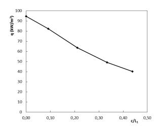
Figure 6. Computation of the net rate at which an infinitesimal element face B gains radiation due to the interaction of the flame in the side a for several values of  $c/L_1$ .
