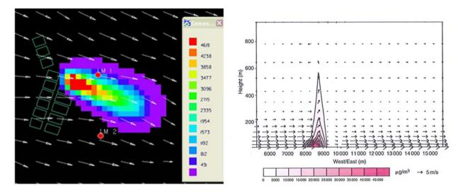
Figure 3. (left) PM10 concentration fields (µg.m<sup>-3</sup>), at ground level, after the burn of three plots (400m x 330m) at GESTOSA 2004 experiments (Valente et al., 2007). (right) Vertical profile of wind and CO concentration in a forest fire in Arrábida (Portugal)(Miranda, 2004).
