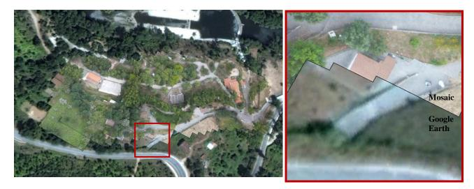
Figure 4. Left: High-resolution mosaic, constructed from aerial images acquired by a quadcopter over the camping site of Côja, overlaying Google Earth. Right: Zoom of the area indicated in red in the image on the left.
